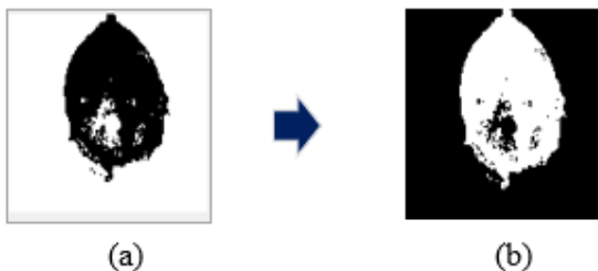
Fig. 4 Image thresholding conversion to binary
